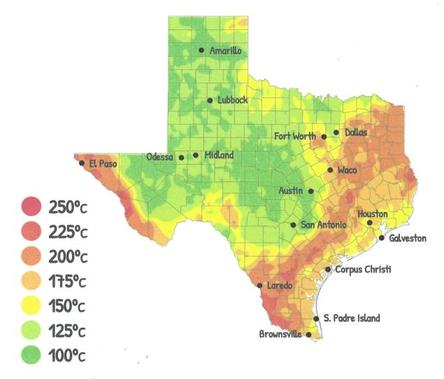
Temperature of Texas geothermal resources at 6.5 kilometers depth. As mapped, much of the State is at or near conventional minimum viable temperatures for geothermal power generation. Source: Adapted from SMU Geothermal Laboratory.
